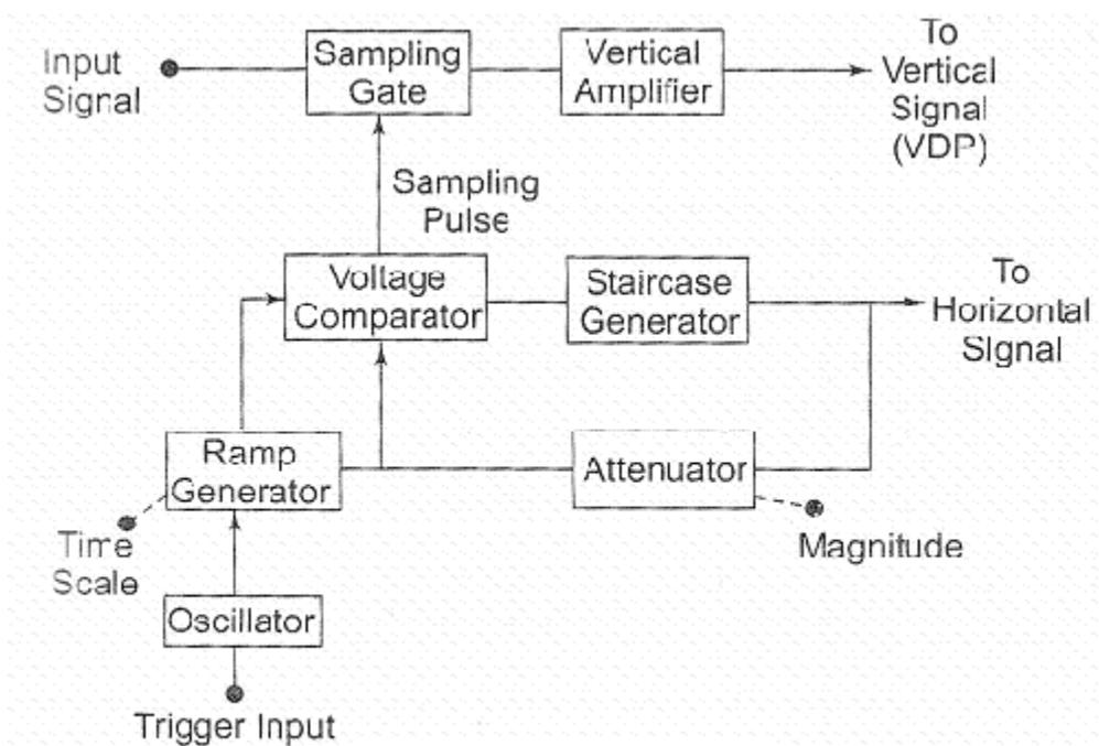
fig 4.1 Sampling Oscilloscope
