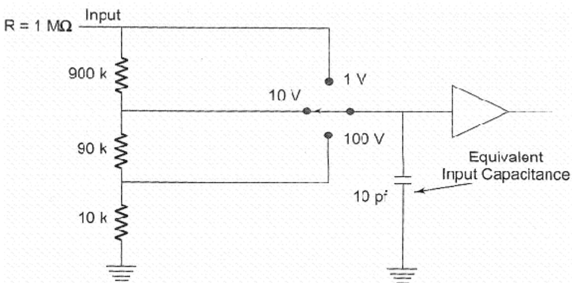
fig 8.1 Uncompensated attenuator
