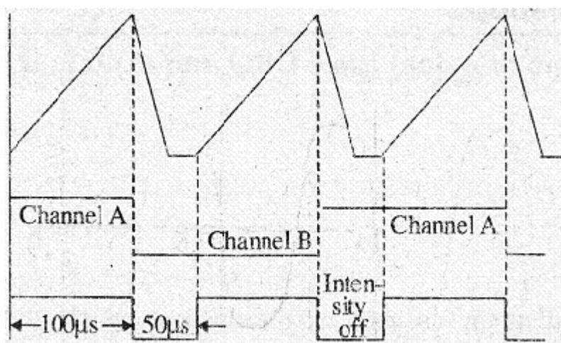
fig 2.2 Wave form of Dual trace oscilloscope in Alternate mode
