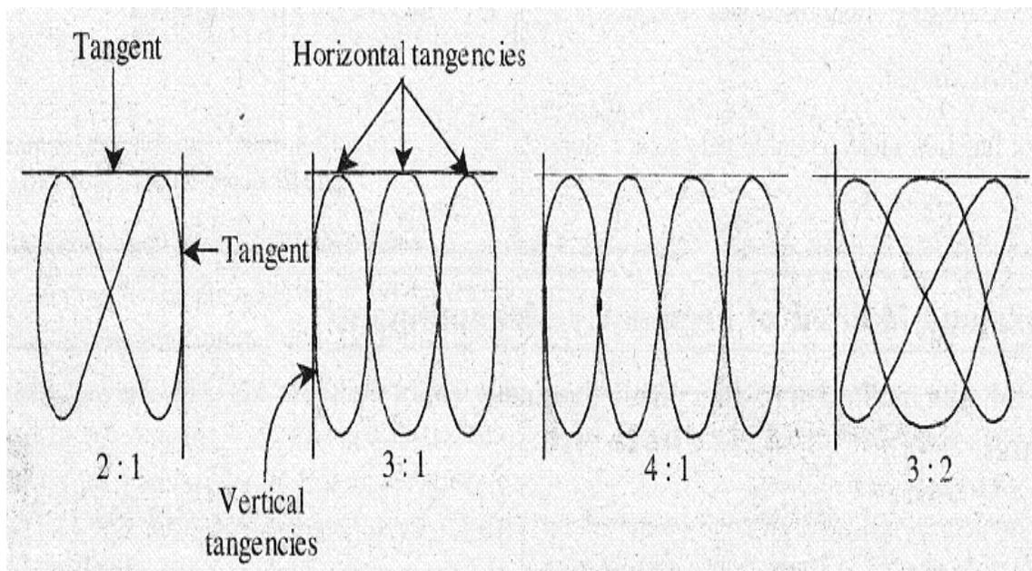
fig 6.2 Lissajous patterns allowing different frequencies ratios
