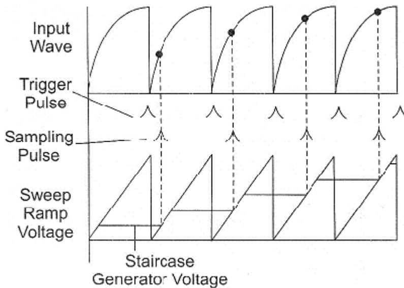
fig 4.2 Various Wave Forms at each block of oscilloscope
