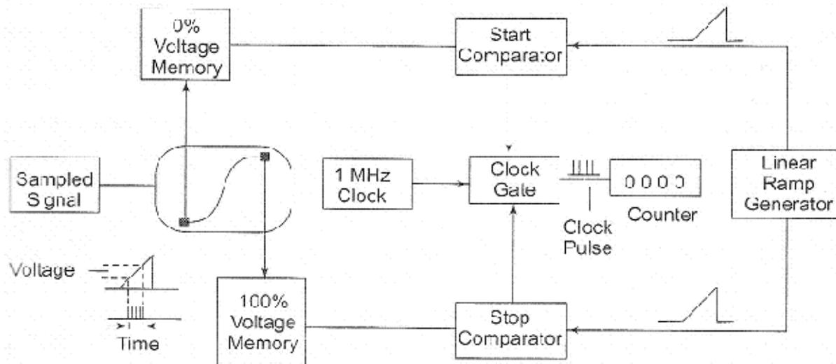
fig 9.2 Voltage to time conversion
