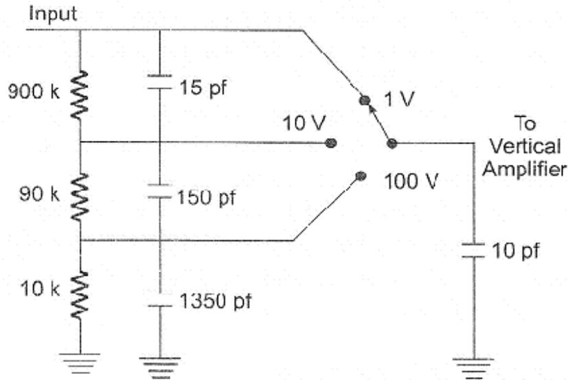
fig 8.2 Simple Compensated Attenuator
