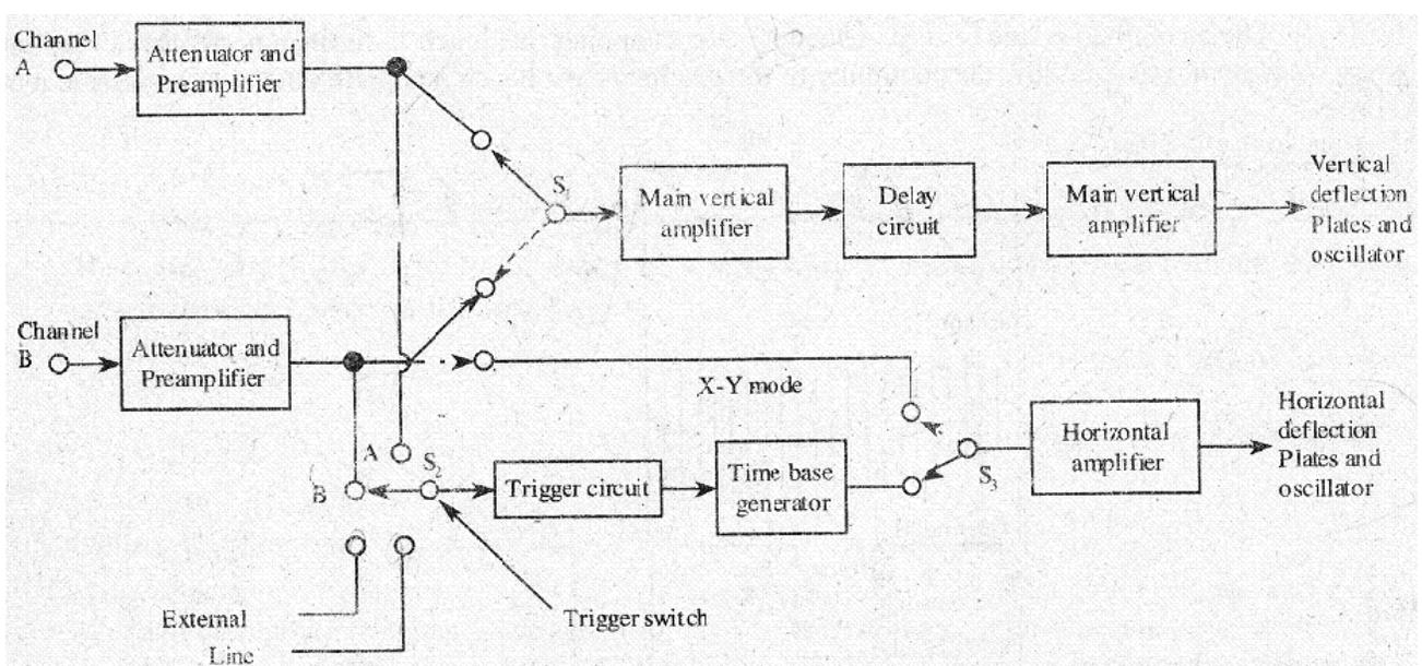
fig 2.1 Block Diagram of Dual Trace Oscilloscope
