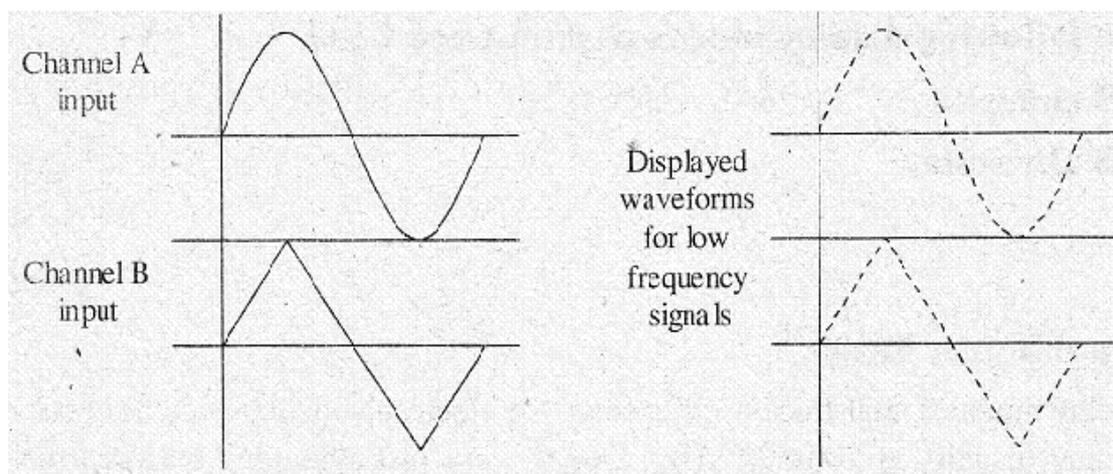
fig 10.2 A and B Alternative mode
