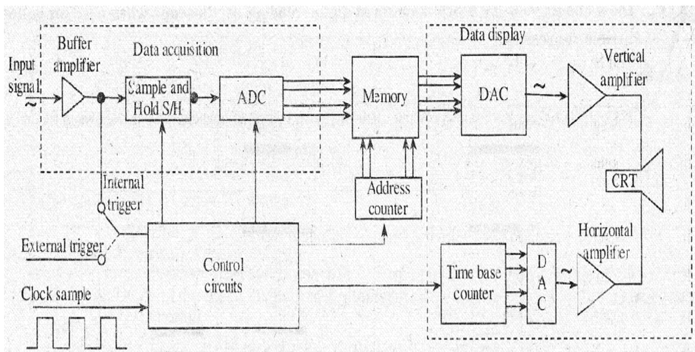
fig 3.1 Block diagram DSO
