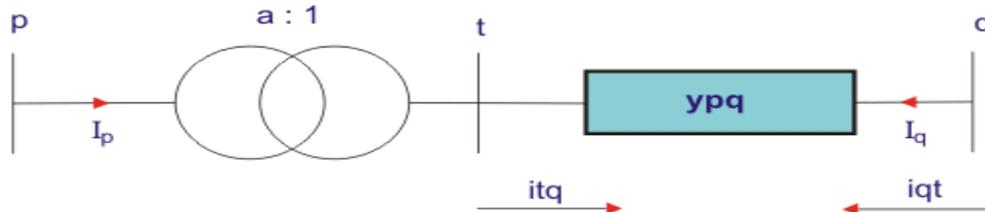
Fig 2: Line Containing an Off Nominal Transformer
