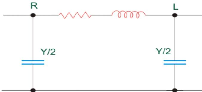
Where,  $R + jX$  is the line impedance and  $Y/2$  is called the half line charging admittance.
