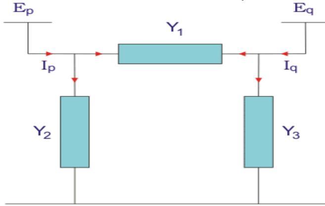
Fig 3: Equivalent  $\pi$  Model of Line
