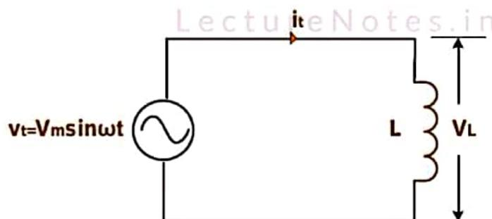
Figure 2.16 Pure Inductor Connected to AC Supply
