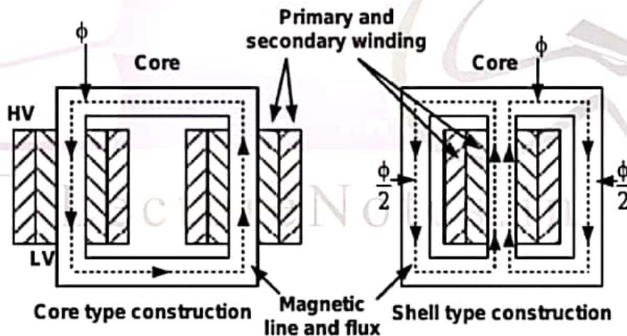
Figure 2.7 Types of construction of 1-phase transformer
