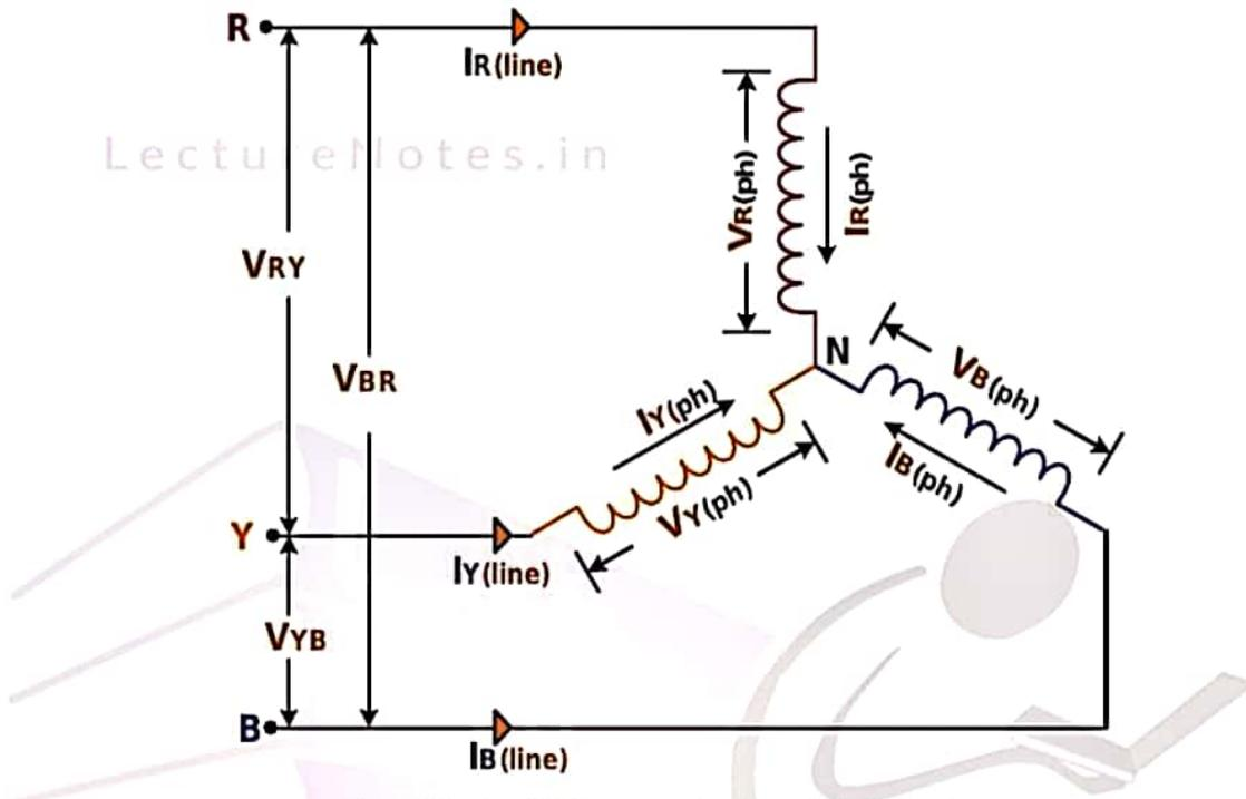
Figure 2.51 Circuit Diagram of Three Phase Star Connection
