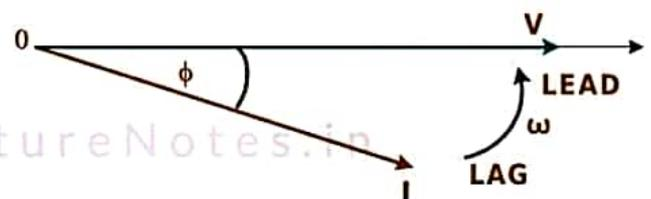
Figure 2.12 Phasor Diagram of Voltage & Current
