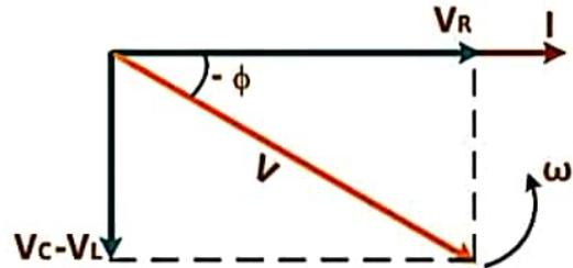
Figure 2.37 Phasor Diagram of Series R-L-C Circuit for Case  $V_L < V_C$
