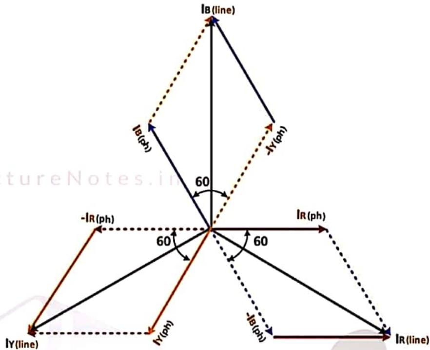
Figure 2.50 Phasor Diagram of Three Phase Delta Connection
