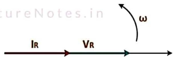
Figure 2.15 Phasor Diagram of Voltage & Current for Pure Resistor
