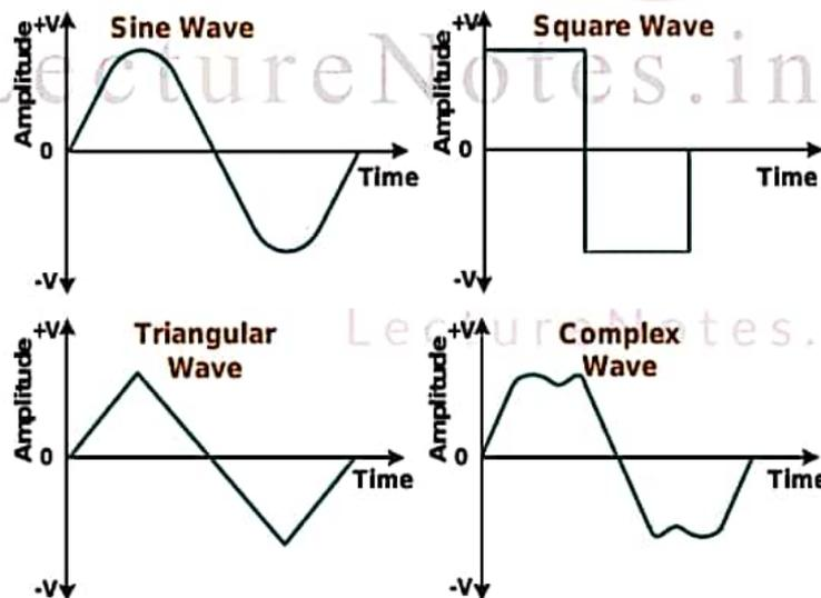
Figure 2.4 A.C. Waveforms
