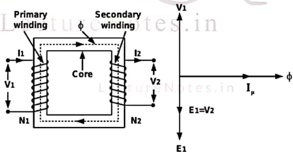
Figure 2.15 Ideal transformer and its vector diagram
