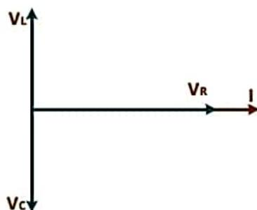
Figure 2.35 Phasor Diagram of Series RLC Circuit
