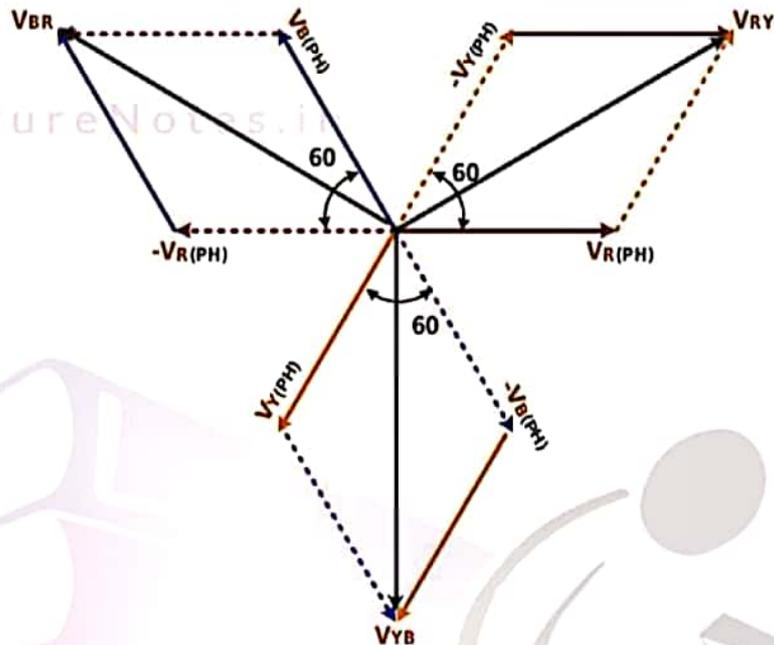
Figure 2.52 Phasor Diagram of Three Phase Star Connection
