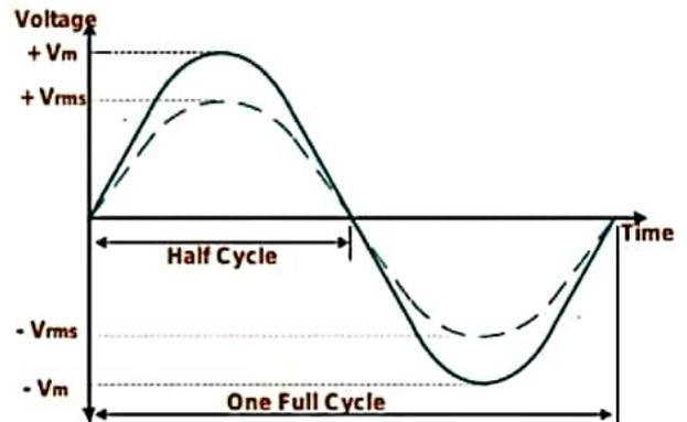
Figure 2.9 Analytical Method for RMS Value
