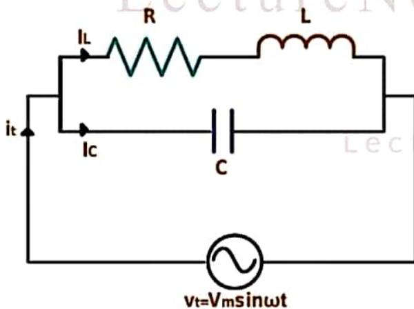
Figure 2.41 Circuit Diagram of Parallel Resonance RLC Circuit
