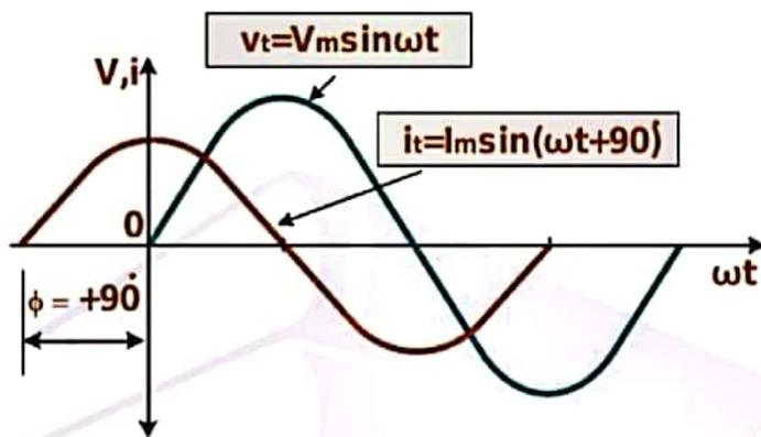
Figure 2.20 Waveform of Voltage & Current for Pure Capacitor
