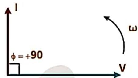
Figure 2.21 Phasor Diagram of Voltage & Current for Pure Capacitor
