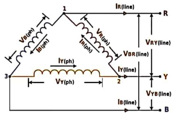
Figure 2.48 Three Phase Delta Connection System
