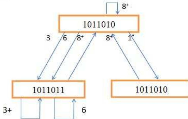
The minimum latency edges in the state diagram are marked with asterisk.
