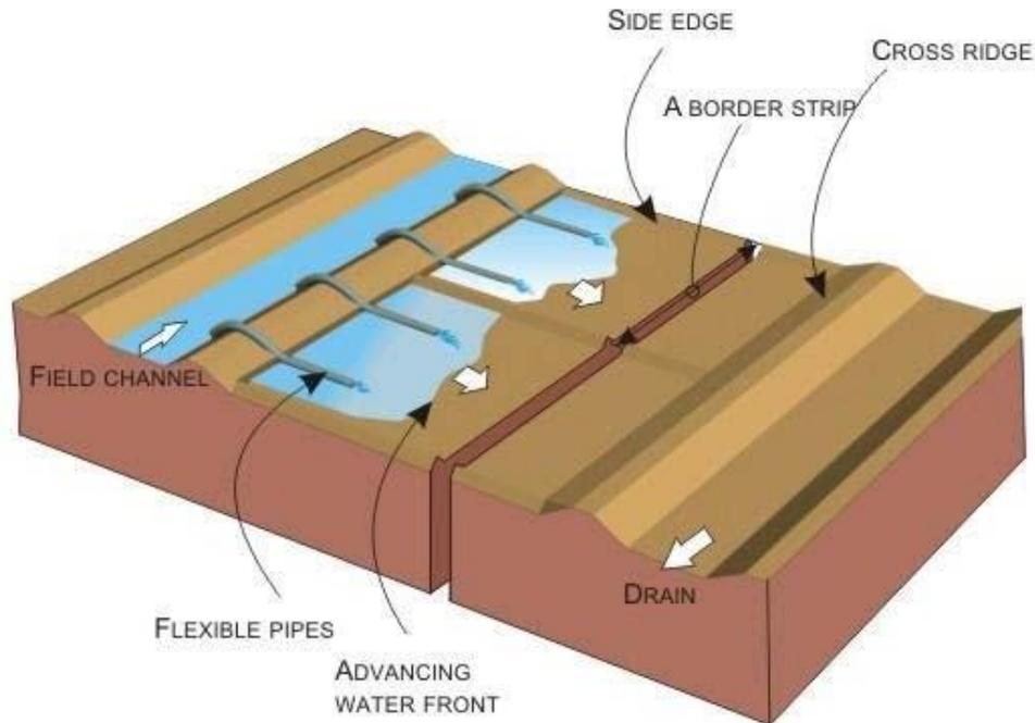
**FIGURE 5. Water entering each border strip independently**
