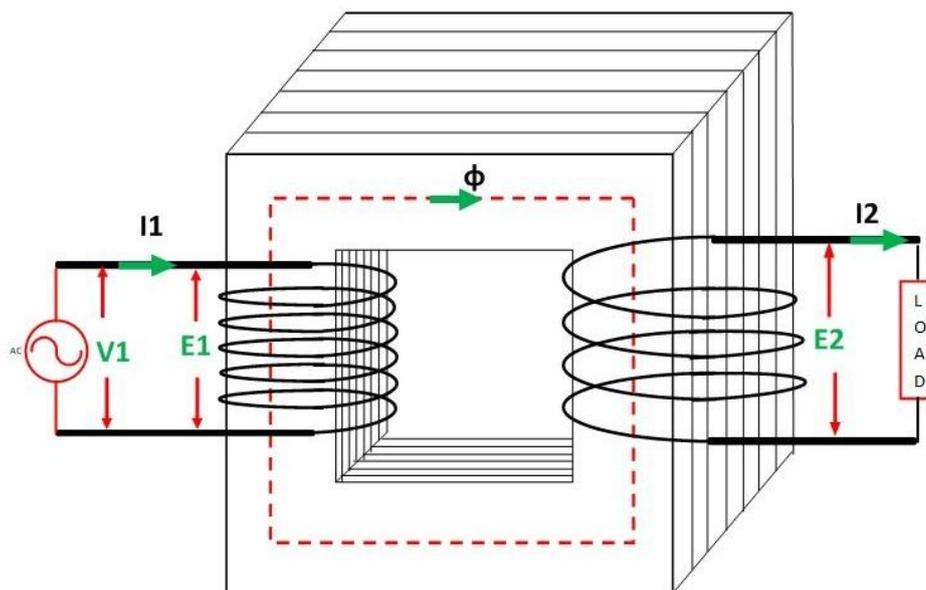
When the AC supply is given to the primary winding with a voltage of  $V_1$ , an alternating flux  $\phi$  sets up in the core of the transformer, which links with the secondary winding and as a result of it, an emf is induced in it called **Mutually Induced emf**. The direction of this induced emf is opposite to the applied voltage  $V_1$ , this is because of the Lenz's law shown in the figure below:
