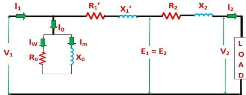
Circuit Diagram of Transformer When All the Primary Quantities are Referred to Secondary Side
