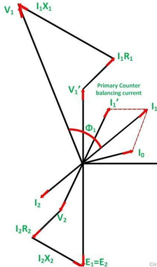
**Phasor Diagram of the Transformer on Inductive Load**
