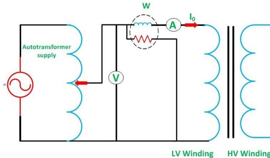
**Circuit Diagram of Open Circuit Test on Transformer**
