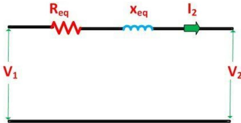
**Simplified Equivalent Circuit Diagram of a Trans**
