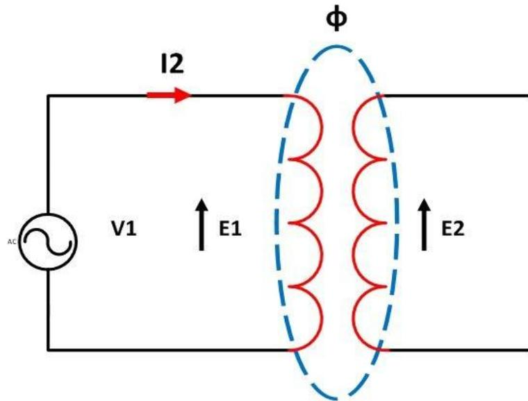
Physically, there is no electrical connection between the two windings, but they are magnetically connected. Therefore, the electrical power is transferred from the primary circuit to the secondary circuit through mutual inductance.
