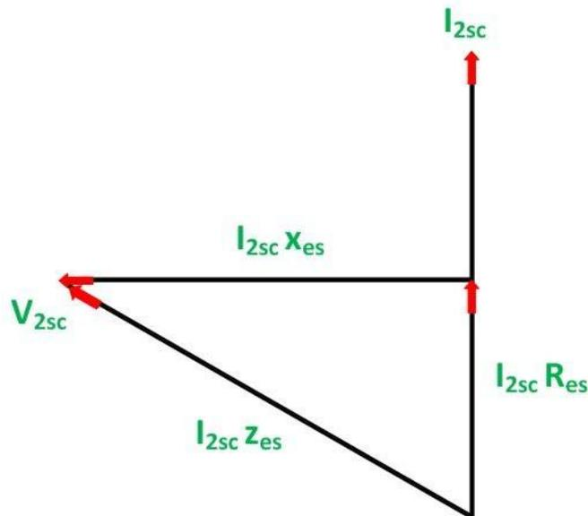
**Phasor Diagram of Short Circuit Test**
