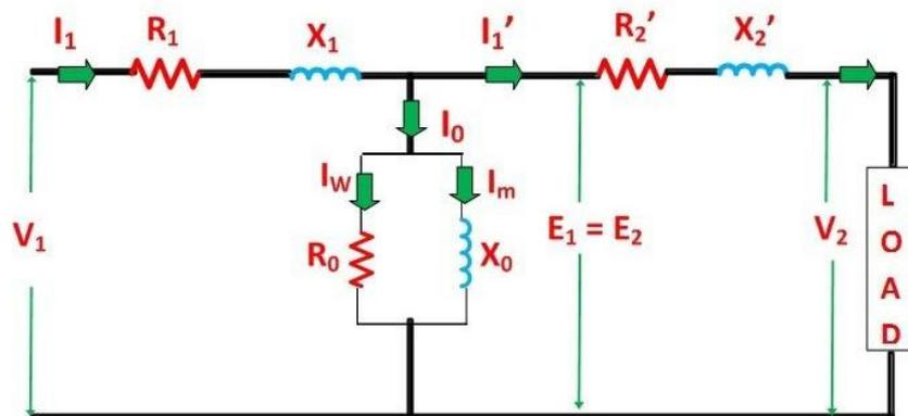
**Circuit Diagram of Transformer when all the Secondary Quantities are Referred to Primary Side**
