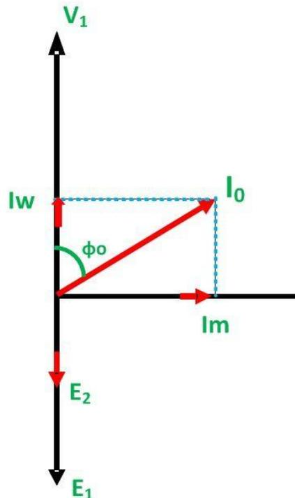
The iron losses measured by the open circuit test are used for calculating the efficiency of the transformer.
