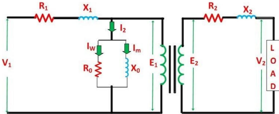
**EXACT EQUIVALENT CIRCUIT DIAGRAM OF A TRANSFORMER**
